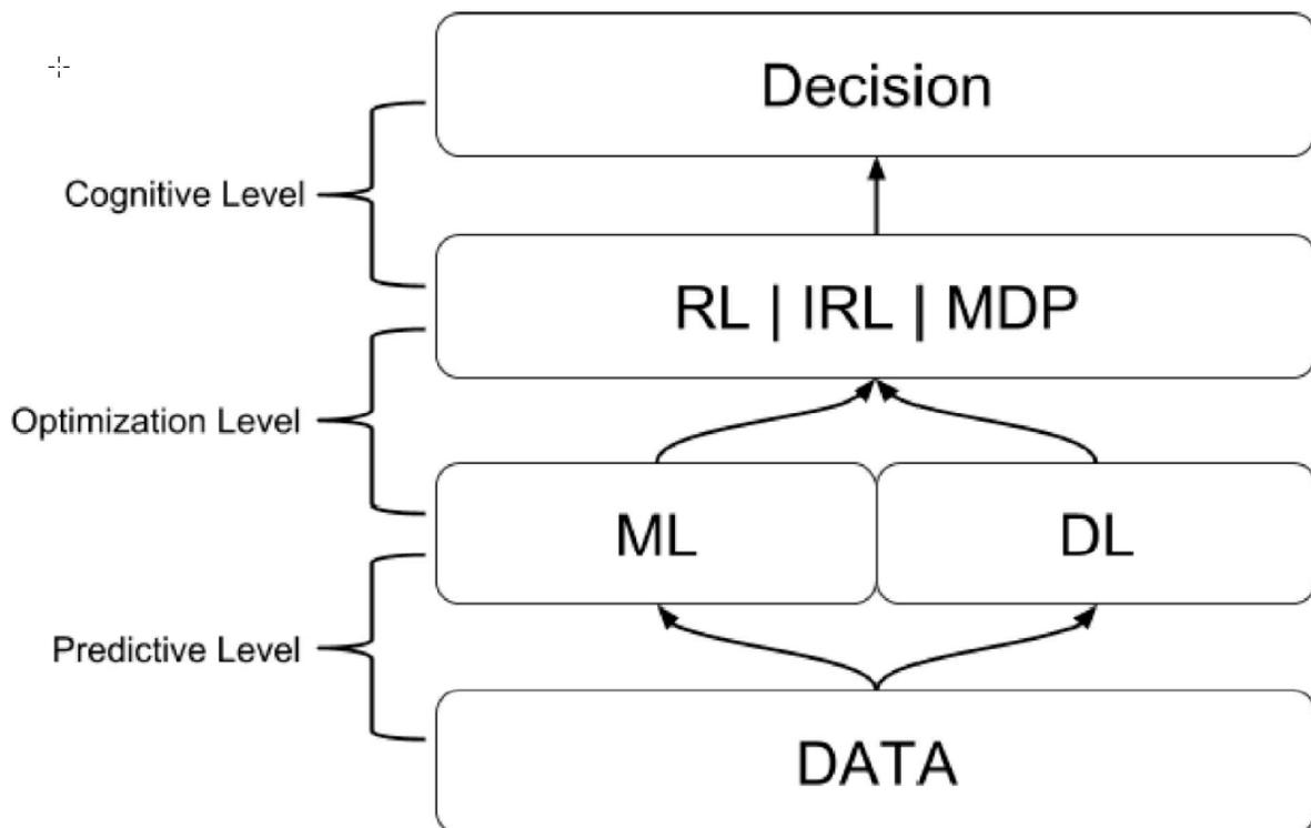
Figure 1. Three levels of artificial intelligence methods in our proposed IDSS.
