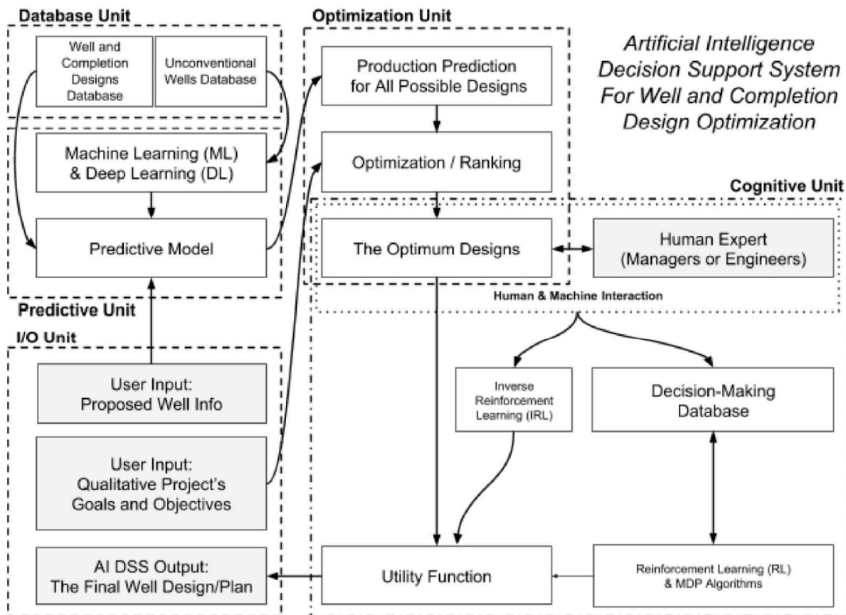
Figure 2. Detailed flowchart of our Intelligent Decision Support System for Field Development Design (a pending patent).
