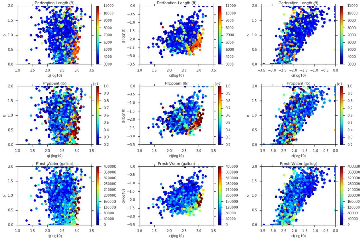
Figure 6. A few completion parameters vs  $q_i$ ,  $d_i$ , and  $b$ .
