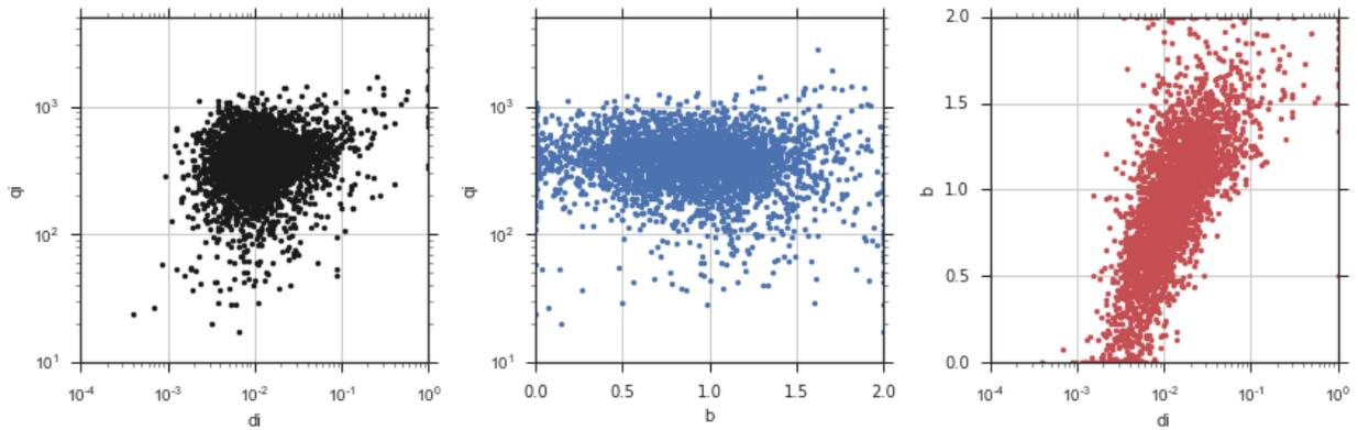
Figure 5. DCA parameters ( $q_i$ ,  $d_i$ , and  $b$ ) for 3541 wells.
