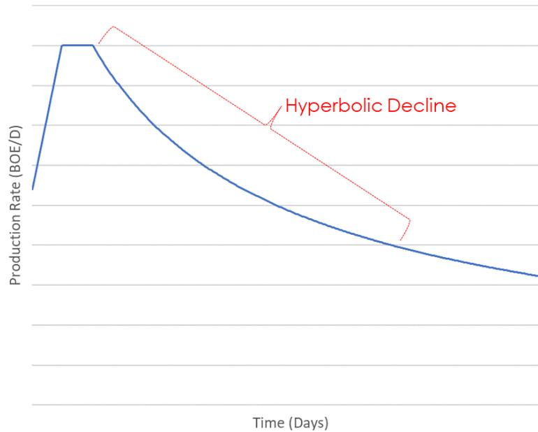
Figure 3. A typical decline curve for the DJ basin wells. In this study, we model the hyperbolic decline part of the curve.
